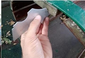
**Finding:** The item has exposed edges and corners with a **Action:** Provide a 3mm radius to all exposed edges and radius of less than 3mm and fails the requirements of BS EN corners 1176
