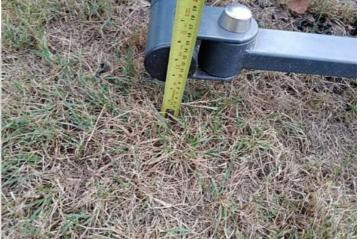
**Finding:** The distance between the underside of the item and the ground is less than the 110mm required by BS EN 16630
