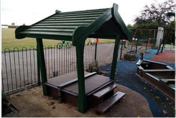
**Finding:** The fence forms a hard object within the impact area of the equipment in contravention of the requirements of BS EN 1176 Part 1
