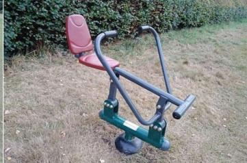
**Finding:** BS EN 16630 - 4.3.1 states that fitness equipment **Action:** Service the item shall be designed so when at rest, the equipment shall automatically adjust so that the equipment is ready for the next user
