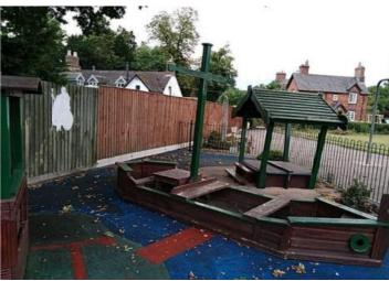
Finding: This item of equipment relies on a single post, or a Action: Ensure that regular detailed inspections are line of posts, for stability and extra care needs to be taken with equipment of this nature to avoid the potential for catastrophic failure
